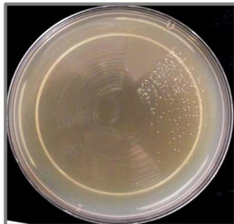
It can be seen that the *S. epidermidis* has been reduced in numbers to undetectable in ~35-40 minutes (the challenge input – nebulizer fluid concentration of the SE#1 was 4.9Log10 and the #1-1 was 4.82Log10) these values show that the inoculums prayed into the chamber are consistent and these plates can be compared to each other for the purposes of efficacy.
